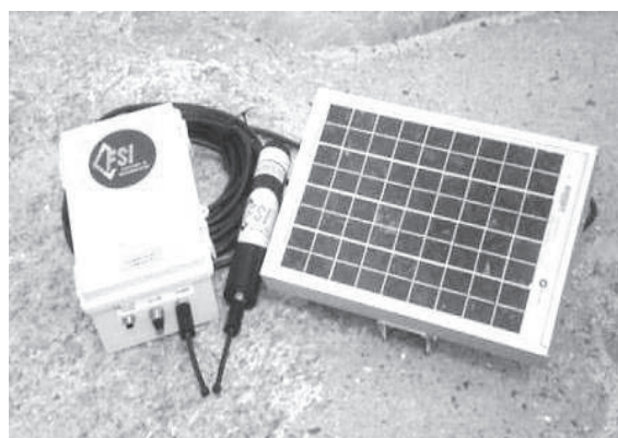
Tide Monitoring System with Optional Solar Charger
